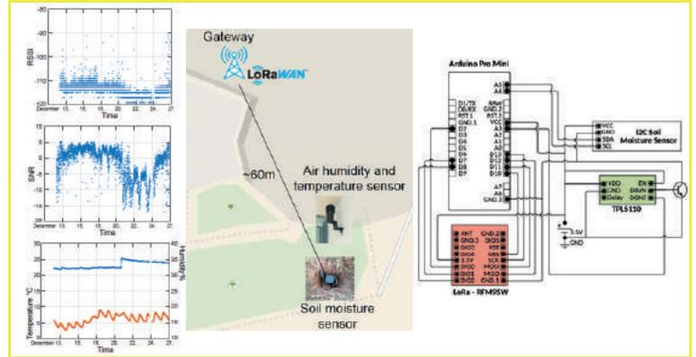
Figure 1. Snapshot of RSSI and SNR signal captured (given in a.) on LoRaWAN gateway (for setup given in b.) from soil moisture sensor, along with I2C sensor measures of soil humidity
