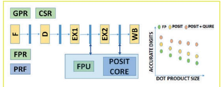
Application-oriented arithmetic (a) posit arithmetic core in a RISC-V processor, (b) accuracy of dot-product using posit and quire
