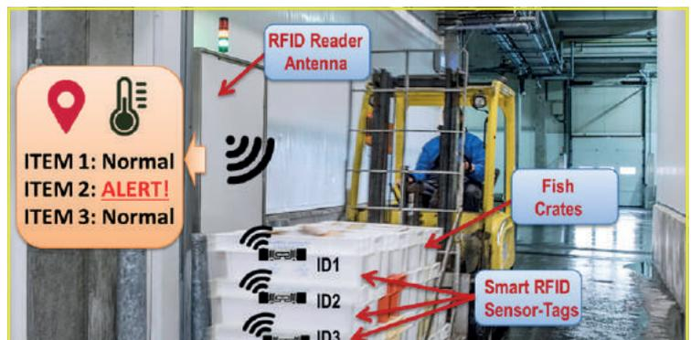
Working principle: once close to an RFID checkpoint, the tags inform the system about the temperature history of the fish boxes.
