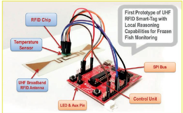
Photo of the first prototype of the C-RFID device realized for validation purposes.
