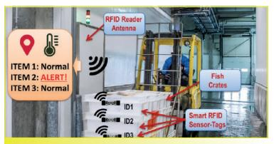
Working principle: once close to an RFID checkpoint, the tags inform the system about the temperature history of the fish boxes.
