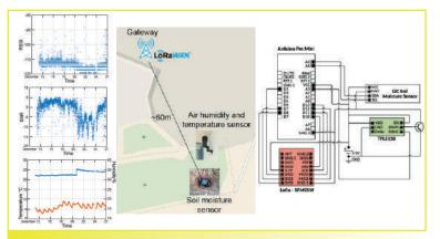
Figure 1. Snapshot of RSSI and SNR signal captured (given in a.) on LoRaWAN gateway (for setup given in b.) from soil moisture sensor, along with I2C sensor measures of soil humidity
