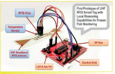
Photo of the first prototype of the C-RFID device realized for validation purposes.
